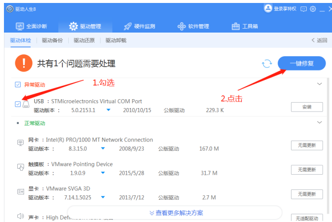
Figure 3.2-2 check "STMicroelectronics virtual COM port" for exception drive and click "one click repair" button
